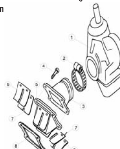
TAV.12 Carburatore e raccordo d' ammissione - Carburettor and and induction pipe - Carburateur et raccord d' admission - Vergaser und Ansaugstutzen - Carburador y racor de admision
