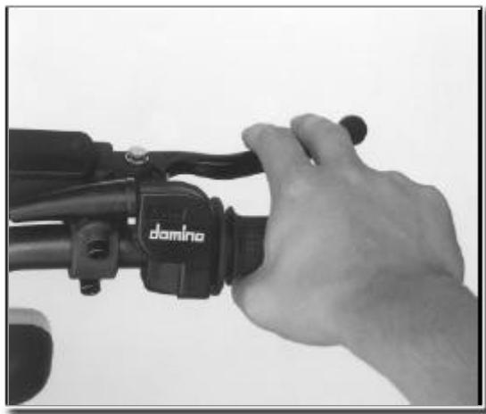
The clutch lever should be set at the necessary distance from the grip and its free play adjusted to maximum of 5mm.
